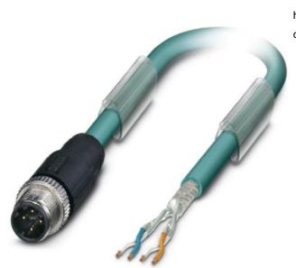
Bus system cable, ETHERNET, 4-pos., PUR blue halogen-free, shielded, straight connector M12 D-coded on free conductor end, length: 10 m
